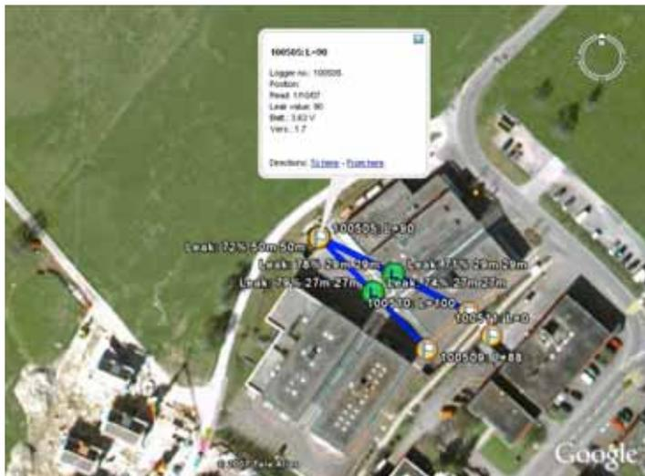
No on-site interrogation or reading of data is required, as the exact leak positions for each project are automatically presented at in the PC software of the Water Loss Manager or nominated PC user. The correlated (pinpointed) leak positions can be displayed automatically within any satellite mapping software running on the users PC.
